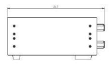
UCL-VA-FS2-1-XX-6-NK variable or step attenuators is programmable attenuator consisting of an double-port input /double-port output test platform, the frequency range DC ~ 6GHz, attenuation range of 0 ~127dB . Through the LCD to reflect the dynamic and static attenuation values, Use the knob to adjust the attenuation values and press to confirm attenuation setting success.
