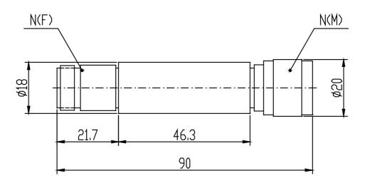
\* Dimensions are given in mm and tolerance  $\pm$ 2%.
